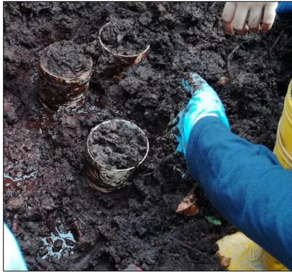
**Figure 2.** Picture of Showing the Undisturbed Sampling Method
